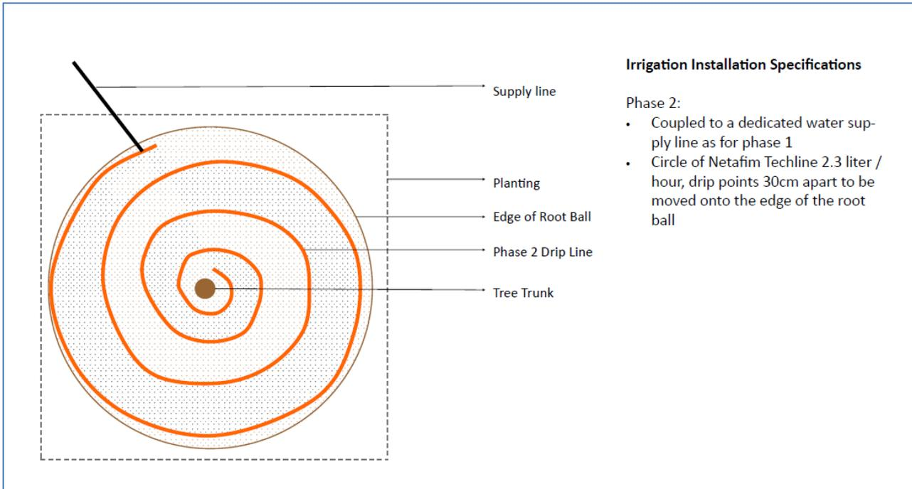
Figure 3 - Diagram of phase 2 irrigation pipe layout
