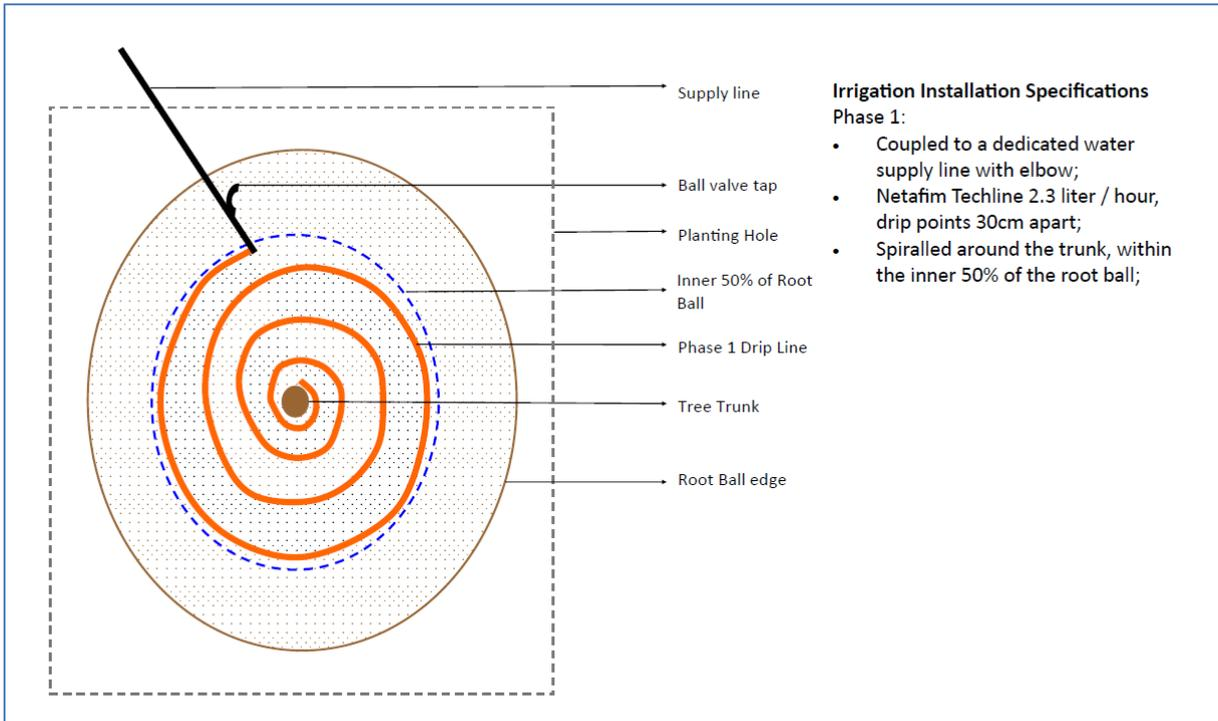
Figure 1 - Diagram of phase 1 irrigation pipe layout
